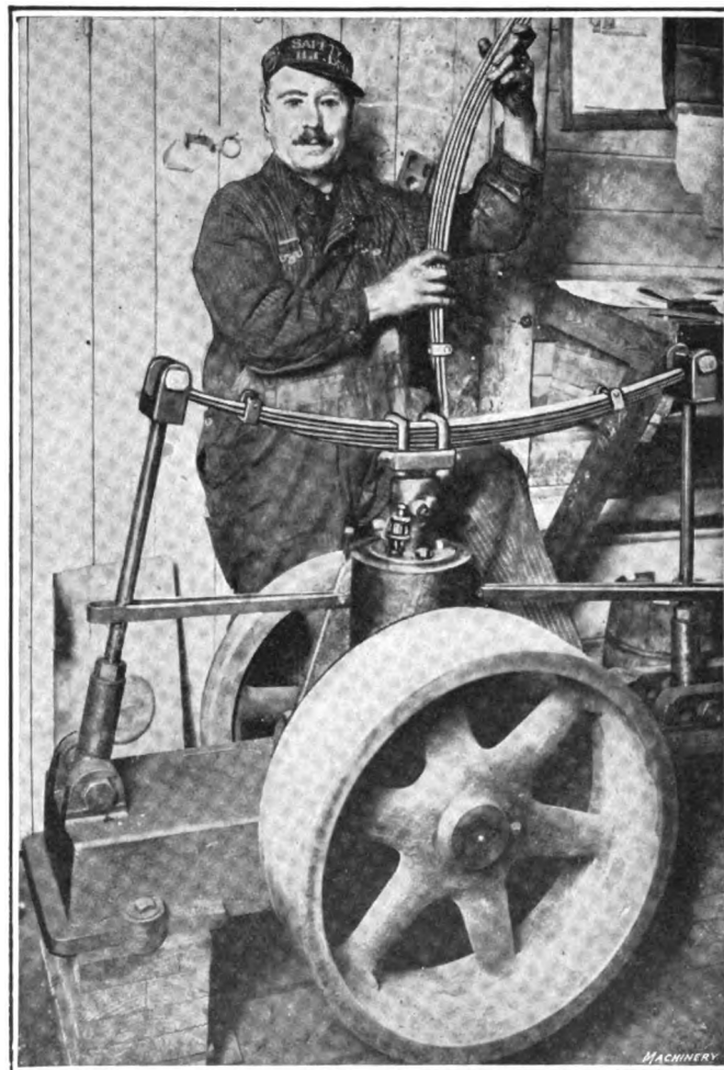
Fig. 5—Vibratory test for automobile springs
